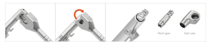
2. Rotate clockwise with a "gear case opener" for removal of the worm gear.
